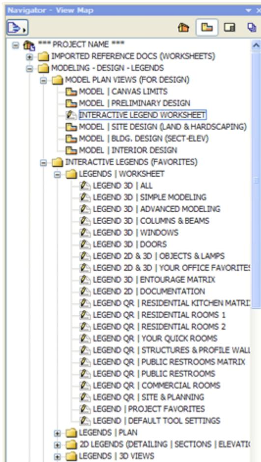
As in AMT 12.1, the preferred method of access to the Legends is through this Worksheet, which uses Virtual Trace to show the Legends from the Plan View. Each saved View in the LEGENDS | WORKSHEET jumps to a specific location or group of parts or Quick Room. This is exactly the same as using the INTERACTIVE LEGEND WORKSHEET View (in the MODEL PLAN VIEWS above) then using the popup menu to zoom to that area of the worksheet.
