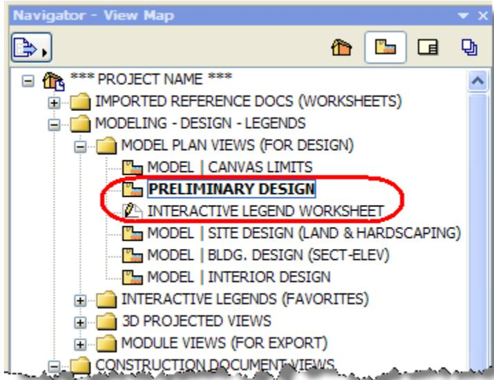
A new Layer Combination called \*PRELIMINARY DESIGN is used for both of these views, so there is no change in layer visibility whether one double-clicks on the Views or uses keyboard shortcuts (F2 for the floor plan, and Last Worksheet / SHIFT+W to go to the Legend Worksheet). Both of these Views are set to ignore the zoom, so you'll always return to the location and zoom where you were looking or working.
